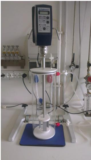
The Rotating cage is an assembly attached to a rotator, whereby a number of corrosion coupons are mounted between two discs. The assembly may be then mounted into a low pressure vessel for rapid screening of corrosion inhibitors or into a HPHT Autoclave for a detailed evaluation. PMAC Rotating Cage apparatus is a complete stand alone set-up, complete with a belt driven stirrer motor, cage for 6 x 2 1/8 " standard corrosion coupons. It has a standard glass cylinder vessel.
