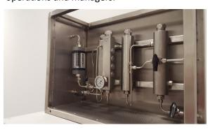
The Field Corrosion Sidestream is designed for dynamic measurement of corrosion rates under flowing conditions, in the absence of online facilities. The standard systems typically operate at pressures of either 100 or 330 bar although a low-
